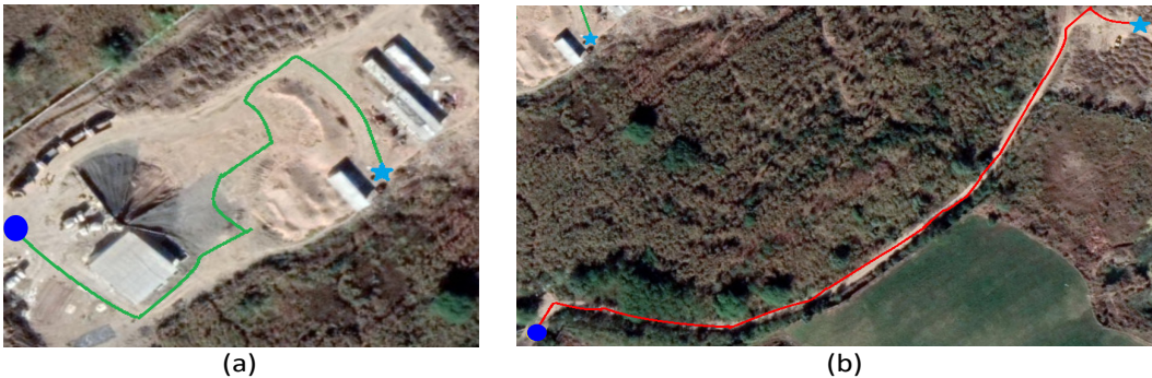
Figure 6: GPS tracks of the vehicle while traversing autonomously in IISER-B campus during testing at two different regions. The terrain included steep climbs, puddles, dynamic obstacles where the vehicle performed robust planning. Blue circle \rightarrow starting location, blue star \rightarrow mission end. The vehicle traversed a total distance of 450 meters in the two tracks.
